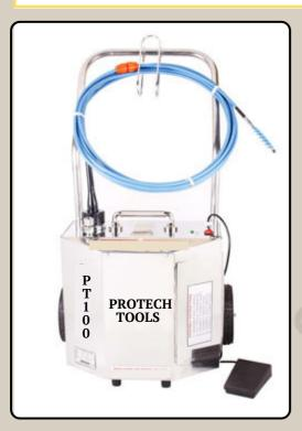
PROTECH TOOLS ELECTRIC TUBE CLEANERS ARE ENVIRONMENT-FRIENDLY COMPACT AND EASILY MENSURABLE UNITS IN HEAT EXCHANGERS, CONDENSERS, BOILERS, AND OTHER TUBE APPAREL THEY WORK BY ATTACHING A CLEANING TOOL (TO BE DETERMINED BY TYPE OF DEPOSIT TO BE CLEANED) TO A FLEXIBLE SHAFT. THE ELECTRIC TUBE CLEANER PROVIDES ROTARY MOTION TO THE FLEXIBLE SHAFT WHICH ROTATES THE CLEANING TOOL INSIDE THE TUBE. IF NEEDED WATER PASSES THROUGH THE FLEXIBLE SHAFT TO AID IN FLUSHING OUT OF THE DEPOSITS.
